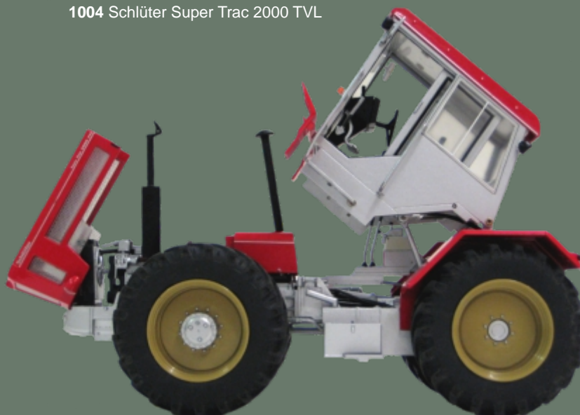
Side-view with opened bonnet, sliding-door and tilted cabin, opened rain cover at exhaust stack.
